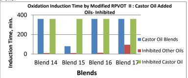
Under severe oxidation conditions of RPVOT as per ASTM D-2272 conditions, all oil blends with castor oils failed to give acceptable levels of induction time. Therefore for high performance applications castor oil blends with low viscosity Gp II mineral oil and a stable ester were explored.
