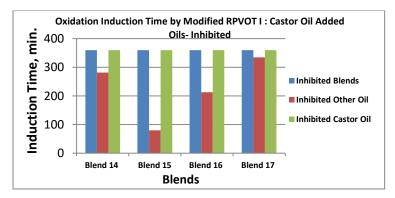
In medium oxidation conditions, inhibited castor oil added blends with other vegetable oils, except soybean oil blend, showed significantly better in thermo-oxidative stability under medium oxidation conditions compared to non-blended inhibited oils.
